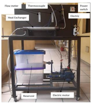
Fig. 2. Schematics of the double pipe heat exchanger.
