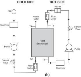
Fig. 1. Sketch of experimental setup (a) Parallel flow (b) Counter flow.
