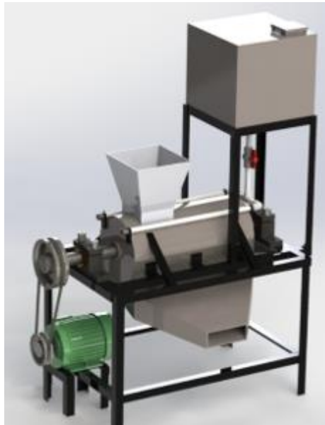
Figure 8. Developed and Optimized Fermented Cassava Mashing and Sieving Equipment
