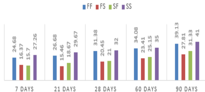
Figure 3: Average compressive strength of concrete cubes at 7, 21, 28, 60, and 90 days, cast and cured with fresh water and saltwater using a water-cement ratio of 0.50.
