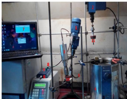
Fig 1. PA6/Carbon Polymerisation set-up.
