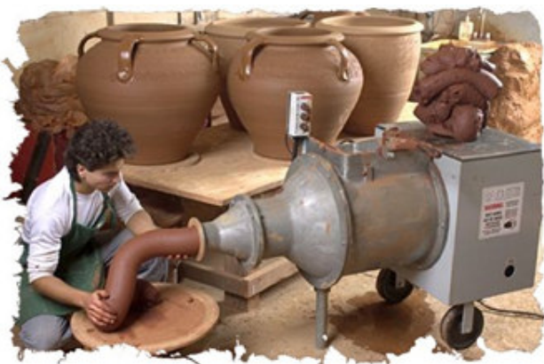
Fig. 2: A ceramist using the pugmill to pug clay for production. Notice the consistency of the pugged clay (out of the pugmill) and the pottery that have been made from the clay. Source: http://www.sheffield-pottery.com/Peter-Pugger-Pugmills-s/45.htm
