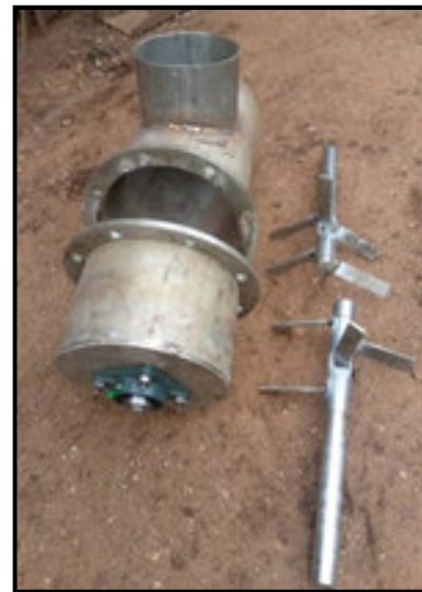
Figs. 9 & 10: The thick stainless-steel halves of the chamber being fabricated. Note the auger assembly.
