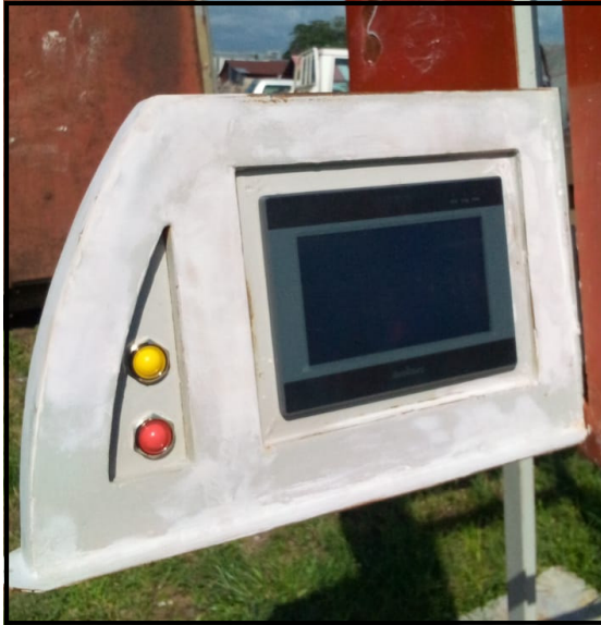
Fig. 7: The retractable touchscreen.
