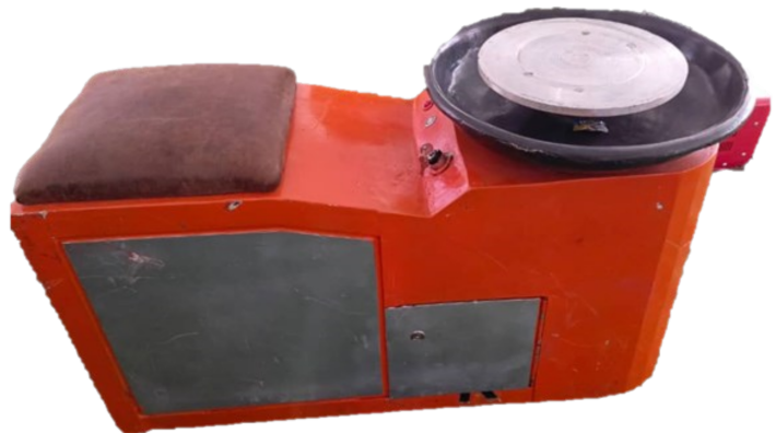
Fig. 4: The redesigned 24VDC throwing wheel
