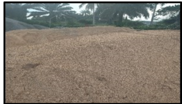
Fig. 4: Fine Aggregate (Source; Sermatech Yard, Odukpani, Nigeria)
